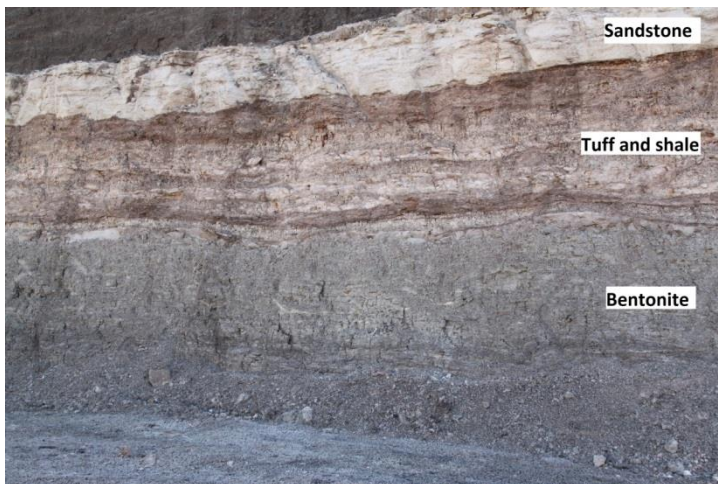
Figure 4 Sodium bentonite (2 metres thick) overlain by tuff and sandstone. Gurulmundi, Australia Source: MTI
