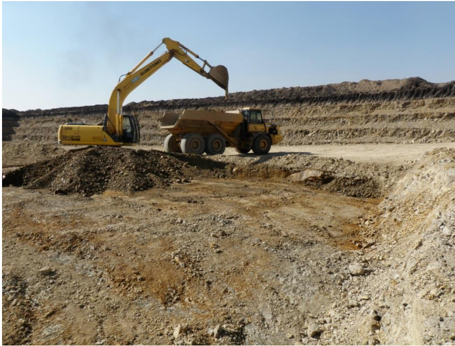
Figure 10 Calcium bentonite being mined from G&W's Blaaubosch pit at Koppies, South Africa Source: G&W Mineral Resources
